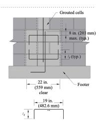
If continuous horizontal reinforcement is not otherwise provided within the end 8 in. (203 mm) of each end of the splice, confinement requirements may be satisfied by providing hooked reinforcement as detailed here. See Tables 4a through 4d for *l*, minimum length requirements. Hook extensions are permitted to overlap.
