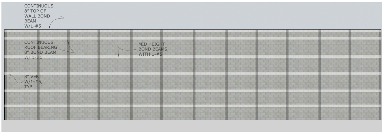
FIGURE 5: WALL WITH BOND BEAMS AND NO JOINT REINFORCEMENT AND NO CJ
