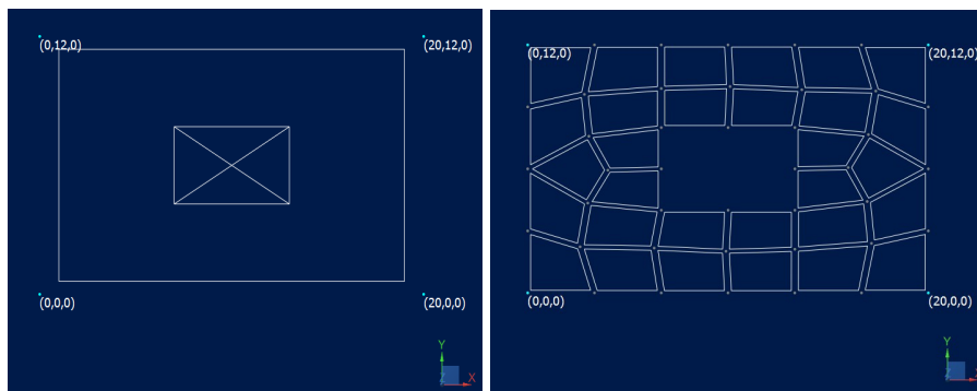
Figure 3: Wall Geometry with opening | Wall discretized into finite elements example of automatic meshing from RAM Elements
