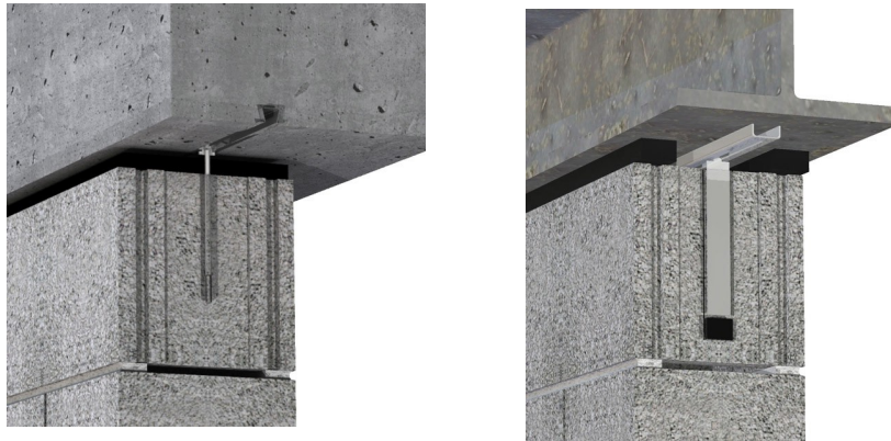
Figure 7: Partition Top Anchors (PTA) source: www.h-b.com
